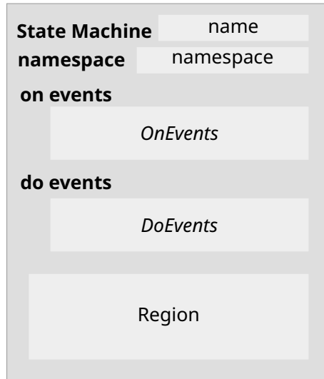
Figure 2.1: Overview of an SMMT Specification
